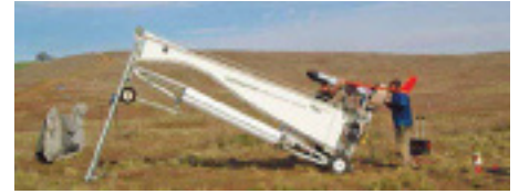
The catapault-launched ScanEagle. Photo by Keith Cunningham appearing Keith's 2014 article for TEAM News, "Robot in the Skies."
